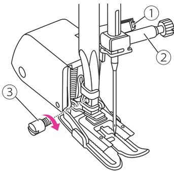
Remove the presser foot holder and attach the walking foot. The lever should be behind the needle clamp screw. Press the walking foot on firmly from behind with your index finger and tighten the screw.
