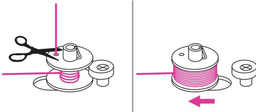
7. After the bobbin has wound a few rounds, stop the machine and cut the thread near the hole of the bobbin. Continue filling the bobbin until it is full. Once the bobbin is full, it rotates slowly. Release the foot control or press the start/stop button to stop the machine, then push the bobbin winder spindle to the left.
