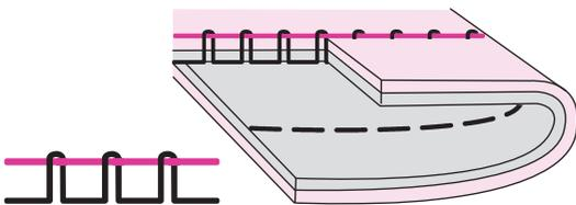
Thread tension is too tight for straight stitch sewing. To reduce the tension, press the "-" button.
