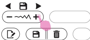
Scroll stitch width adjustment button "+" or "-" repeatedly, the LCD will display the stitches and the settings that have been stored one by one.
