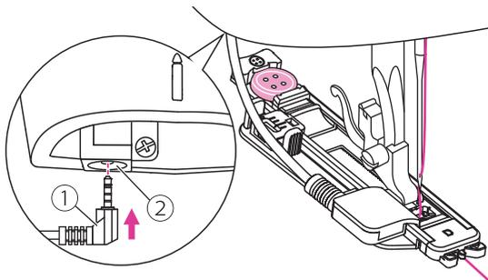
Attach the electronic buttonhole foot and plug the cord into the socket above the presser foot bar.
