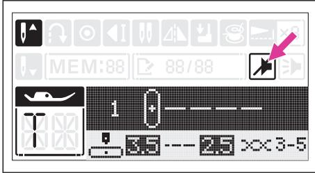
Buzzer turn on: When machine is in silent mode, press the button for 2 seconds and it will deliver two short beeps to remind you that the sound is turned on now.
