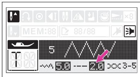
Press the stitch length adjustment button "+" or "-" to adjust the stitch length. Neat zigzag stitches are usually achieved at "2.5" or below.
