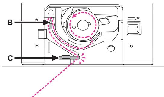
Pull the thread through the slit (A).
