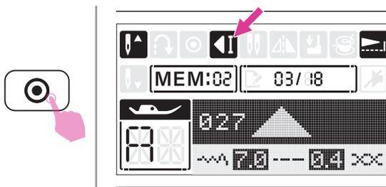
During machine is sewing, the machine will sew 3 locking stitches at the end of the current stitch if the auto-lock button pressed. Then it will stop automatically. The LCD screen will display the auto-lock icon. If pressing the start/stop button again, it will sew from the next stitch.
