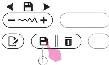
Press the memory button to save the stitches combination, and return to standard sewing mode. Recall the memorized stitches and start to sew.
