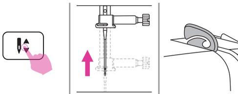
2. Press the needle up/down position button to bring the needle and take-up lever to highest position.
