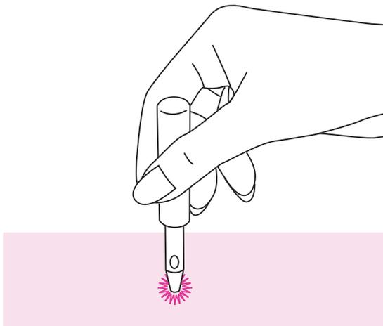
Make a hole at the center using an eyelet punch.
