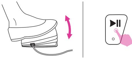
7. Slowly press down the foot control or long press the start/stop button to start sewing. Release the foot control or press the start/stop button again to stop the machine.
