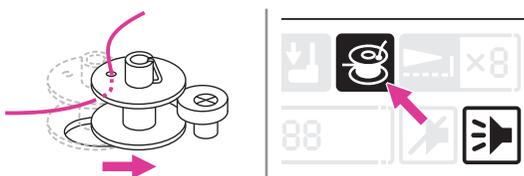
5. Push the bobbin to the right. When the bobbin winder spindle is pushed to the right, the screen will display the icon.
