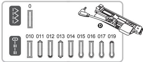
Using the electronic buttonhole foot.
