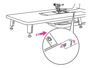
Snap (A) of the extension table into (B) of the machine.
