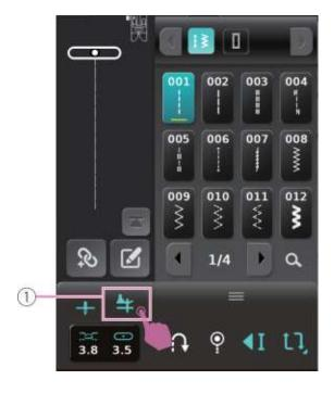
When you want to change the sewing direction, you can also set the pivot function in the sewing mode. When you stop sewing, the needle will stay in the fabric, and presser foot will automatically lift, which can easily rotate the fabric. This function is very useful. (Presser foot height setting, please refer to "setting" chapter for more information.)
