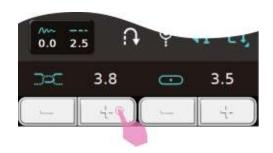
Press the "+" or "-" button to adjust the stitch tension.
