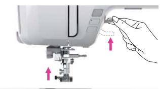
When sewing multi-layers or thick fabrics, the presser foot can be further raised up manually to allow enough space for your sewing work.
