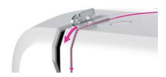
5. Continue to guide the thread into the silver discs to keep the thread in proper tension.
