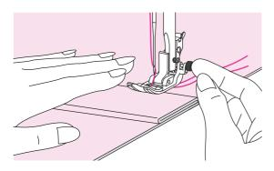
When you reach the point of an increased thickness, lower the needle and raise the presser foot lifter. Press the toe of the foot to the horizontal line and push in the black button, then lower the foot and continue sewing.
