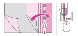
Turn the fabric right side out. Attach the left pin for sewing the rightside of the zipper.
