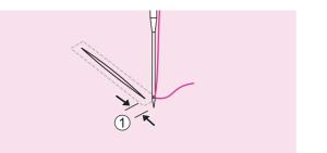
Position the fabric so that the needle is 2mm in front of the area to be darned, and then lower the presser foot lifter.
