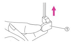
Raise the presser foot lifter and cut the thread. To sew over the same buttonhole, raise the presser foot lifter (it will return to its original position).
