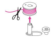
Hold the thread tail securely in one hand. Step on the foot control or press the start/ stop button to start winding the bobbin.
