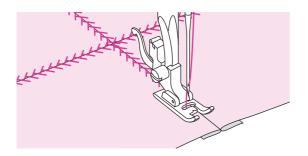
Working on the right side of the fabric, place the center of the presser foot on the seam line of the joined fabrics and stitch over the seam.
