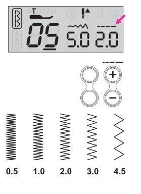
Press the stitch length adjustment button "+" or "-" to adjust the stitch length. Neat zigzag stitches are usually achieved at "2.5" or below.
