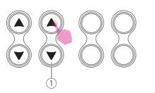
Press stitch selecting buttons adjustment up or down for right digit position between  $0\sim9$ .
