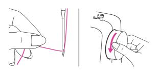
Hold the upper thread with your left hand. Turn the handwheel towards you (counterclockwise) to lower the needle down below the needle plate then raise it to bring the bobbin thread up.
