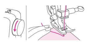
clockwise) to lower the needle into the fabric at the beginning of the stitching.
