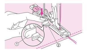
Pull the buttonhole lever all the way down and position it behind the bracket on the buttonhole foot.
