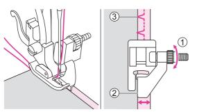
Place the fabric under the foot. Turn the handwheel forwards until the needle swings fully to the left. It should just pierce the fold of the fabric. If it does not, adjust the stitch width accordingly. Adjust the guide by turning the knob so that the guide just rests against the fold.
