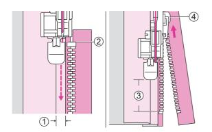
Attach the zipper foot. Attach the right pin for sewing the left side of the zipper. Sew the zipper to the piece of fabric with the extra 3mm, starting from the end of the zipper.
