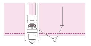
Position the fabric under the presser foot so that the centerline's mark is aligning with the center of the buttonhole foot.
