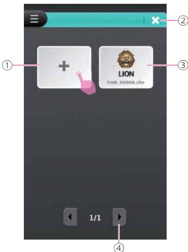
Click Add icon to save the pattern, after saved the pattern, the screen will go back to the edit page. The saved pattern will save in order. If you want to save the new pattern by replacing the existing file, click the existing pattern and confirm the warning message.
