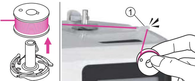
8. Remove the bobbin then use the thread cutter on the right side to cut.
