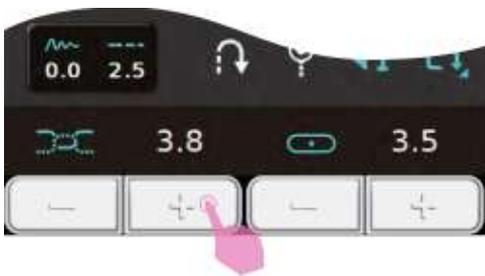
Click the Thread tension icon and a slider will pop out for quick value adjustment. Click anywhere on the screen to leave the window. Click the Thread tension value icon will reset the value to default.
