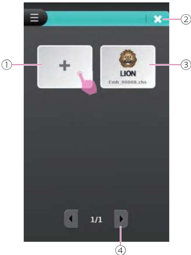
Click Add and save pattern icon to save the pattern, after the pattern saved, the screen will go back to the edit page. The saved pattern will be shown in order. If you want to save the new pattern by replacing the existing file, click the existing pattern and confirm the warning message.
