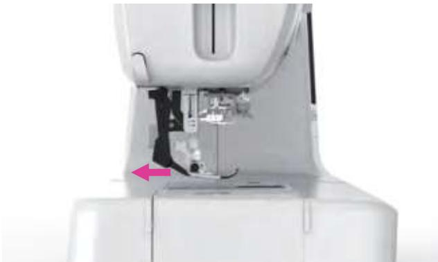
Pull down the DFS mechanism and swing it to the rear to disengage.
