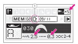
The stitch length, stitch width, mirror and elongation of the stitches can be adjusted manually depending on each stitch settings.
