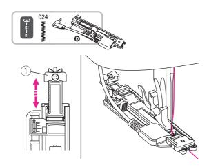
Using the electronic buttonhole foot.
