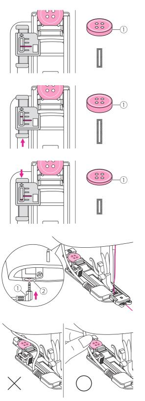
The red mark is the standard setting for regular button, adjust the pointer align with the red mark.
