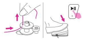
Hold the thread tail securely in one hand. Step on the foot control or press the start/ stop button to start winding the bobbin.
