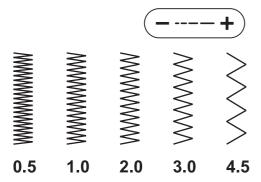
Press the stitch length adjustment button "+" or "-" to adjust the stitch length.
