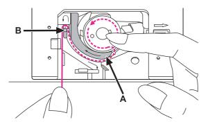
With a finger hold gently on top of the bobbin, please follow the arrow markings and draw the thread into the bobbin thread guide from (A) to (B).
