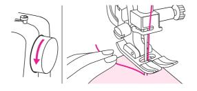
5. Turn the handwheel toward you (counterclockwise) to lower the needle into the fabric at the beginning of the stitching.
