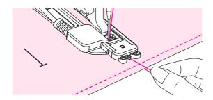
Slightly hold the end of the upper thread and start sewing. Pull two lines together.
