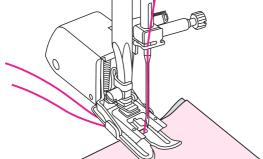
Draw the bobbin thread up and place both bobbin thread and needle thread behind the walking foot attachment.
