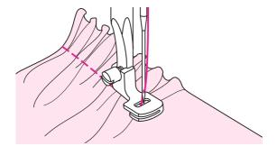
Remove the presser foot holder and attach the gathering foot, set the tension below 2. Place fabric to be gathered under presser foot to the right of the presser foot.
