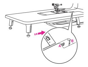
Snap (A) of the extension table into (B) of the machine.
